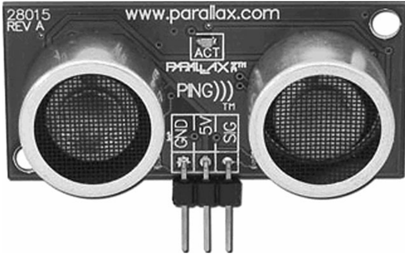
FIGURE 17.8 The Ping))) ultrasonic sensor determines the distance to objects in the robot's path.
