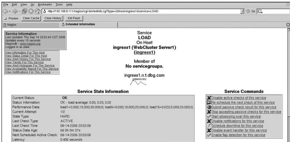
Figure 7.23 Sparkline embedded into the Nagios Web interface.
