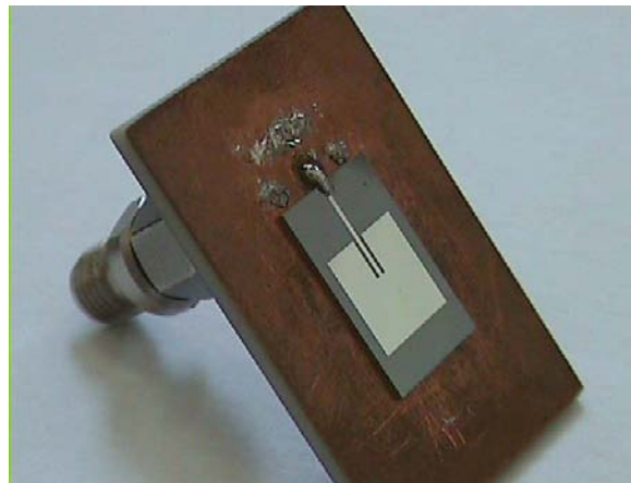
Figure 13. A 7.7 \times 7.6 \text{ mm}^2 patch antenna realized on a HRS substrate ready for reflection measurements.
