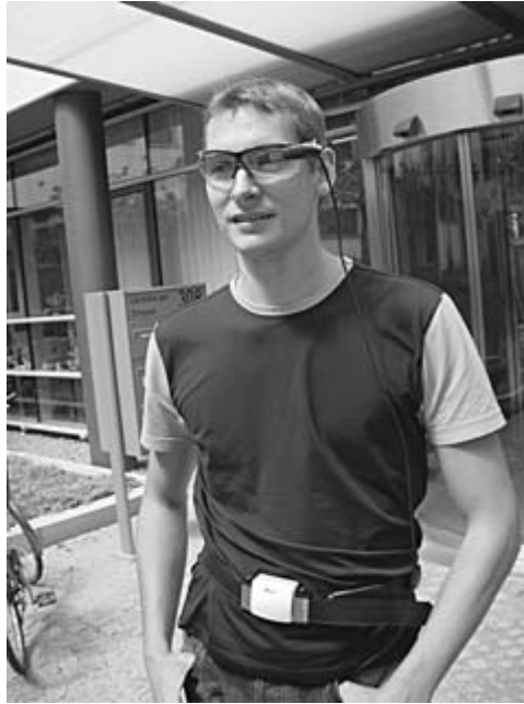
Figure 2-12. Wearable computer integrated in a belt and attached to head-mounted display
