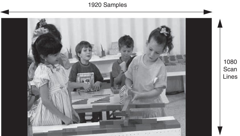
FIGURE 5.14 Scaling 4:3 Content for a 16:9 Display: “Normal” mode. Left and right portions of 16:9 display not used, so made black or gray.
