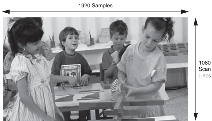
FIGURE 5.16 Scaling 4:3 Content for a 16:9 Display: “Zoom” mode. Top and bottom portion of 4:3 picture deleted, then scaled to fill 16:9 display.
