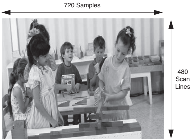
FIGURE 5.12 Scaling 16:9 Content for a 4:3 Display: “Squeezed” mode. Entire 16:9 program horizontally squeezed to fit 4:3 display, resulting in a distorted picture.
