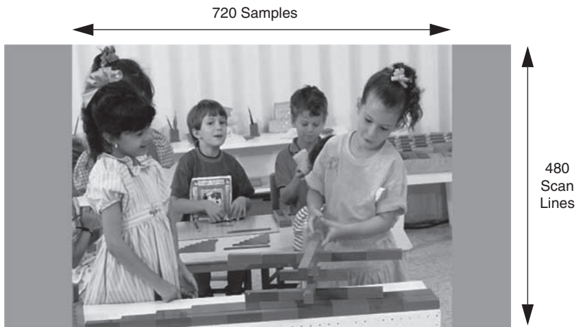
FIGURE 5.10 Scaling 16:9 Content for a 4:3 Display: “Normal” or pan-and-scan mode. Results in some of the 16:9 content being ignored (indicated by gray regions).
