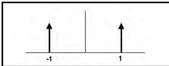
FIGURE 1.1 The Probability Distribution of a Square Wave Has Only Two Values
