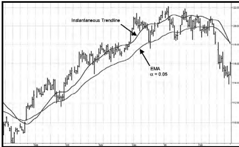
FIGURE 2.7 Instantaneous Trendline Has Much Less Lag than an EMA ( \alpha = 0.05 )
