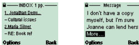
Fig. 4. Examples of a WAP e-mail list and message screens. On the left, the list, and on the right, the message.
