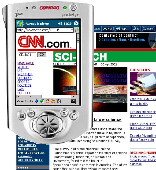
Fig. 1. A Web page with a complex design, as seen on a Pocket PC. The original page width is three times the width of the Pocket PC display
