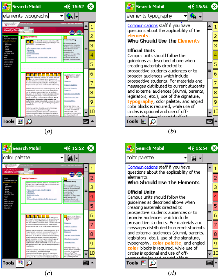
Fig. 4. The SearchMobil booklet interface showing documents in the context of a set of search results: (a) result 4 of a global search for “elements typography”; (b) a selected segment from this page, with highlighted query terms; (c) a local search over the original result set, for “color palette” (the tabs of relevant pages have changed colour), showing the new term hits; (d) the same segment as in (b) with the new query terms highlighted
