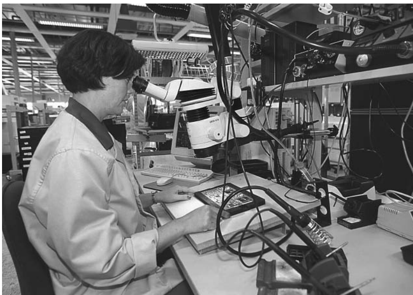
A microelectronics technician at an Ericsson mobile phone factory uses a microscope to check mobile phone circuits. (Alex Farnsworth, The Image Works )
