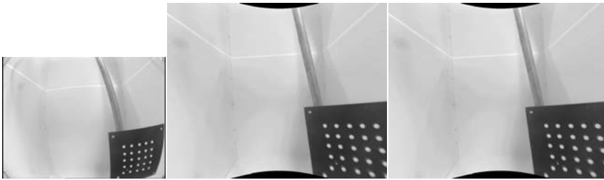
Figure 1.19. Distortion: (a) original view ( 768 \times 576 pixels), (b) non-distorted view ( 968 \times 776 pixels) from data obtained in water; (c) non-distorted view from data predicted from air
