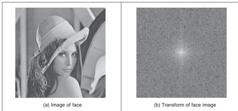
Figure 2.16 Applying the Fourier transform to the image of a face
