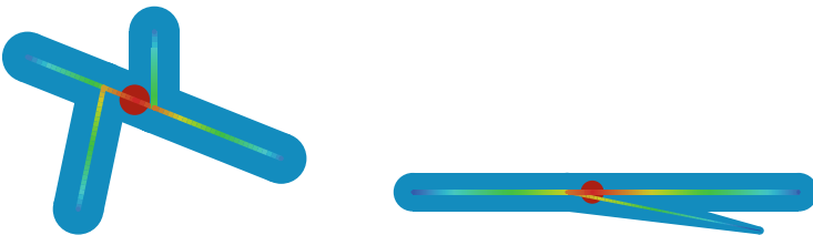
Fig. 9.10 The medial axis of two shapes, the EDF along the medial axis (in color), and the EMA (red dot)
