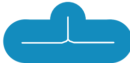
Fig. 9.7 The medial axis (in white) for a shape (in blue). The junction in the medial axis indicates a branching, which is a criteria for identifying shape features
