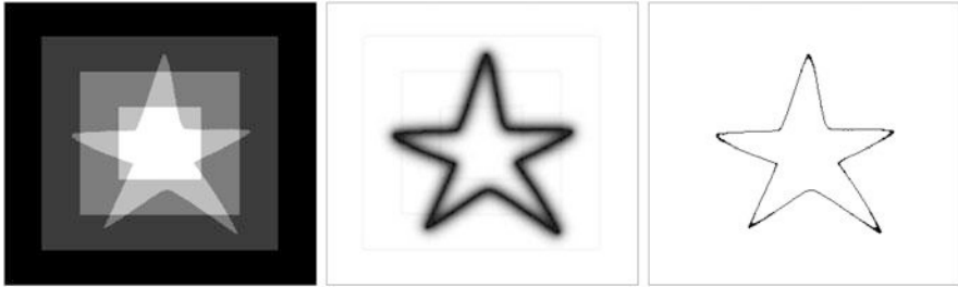
Fig. 1.3 From left to right: the input image which has a star occluded partially by the background, the output edge strength function v , and the extracted boundary
