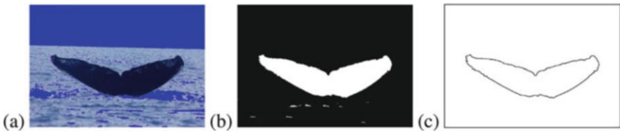
Fig. 6.1 Intermediate steps for extracting the medial axis from the whale image. The original image can be seen in Fig. 6.6. Images above are (a) the initial cluster containing the whale fluke resulting from k -means clustering, (b) the segmented whale fluke after morphological processing, and (c) the resulting boundary points. The medial axis with longest path resulting from the boundary displayed here can be seen in Fig. 6.2e
