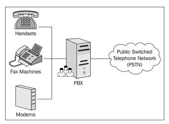
In the previous diagram, each extension (meaning everything to the left of the PBX) can connect to any other extension by dialing it directly. This means if a modem were to send a fax to a local fax machine, it would be done by creating a direct connection between the devices through the PBX.
