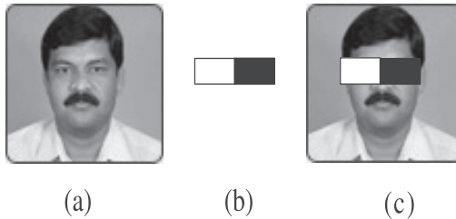
FIGURE 4.4: Application of Haar feature on given image
