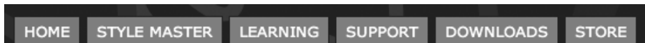
Figure 3-10. An elegant navigation menu, created with nothing more than an unordered list and some CSS
