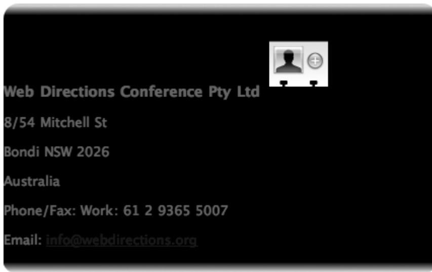
Figure 7-19. With the second bottom border image added, the rounded corners are finished.
