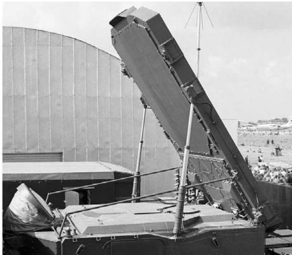
Figure 7.2 Tombstone space-fed lens array used in Russian SA-20 SAM system.
