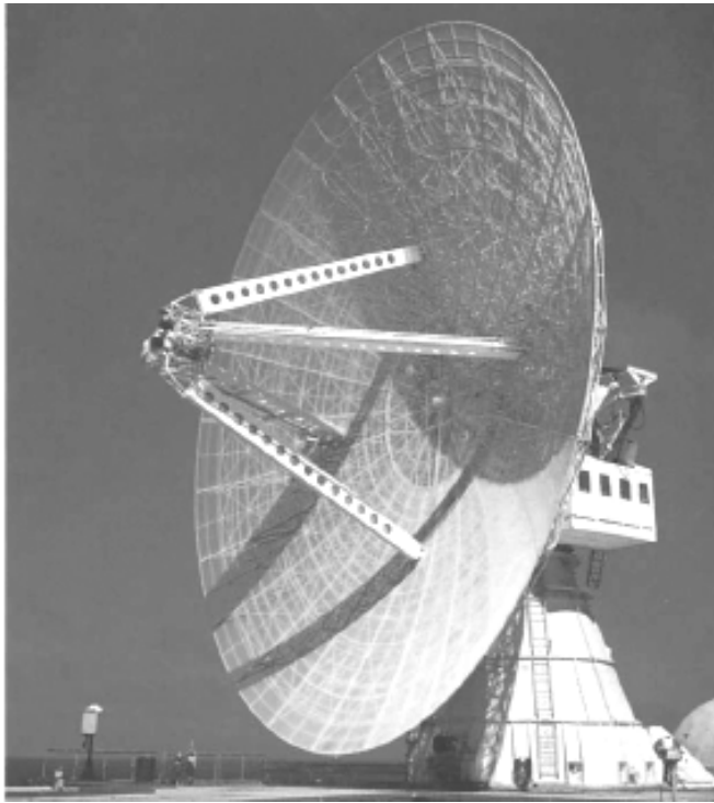
Figure 13.1 TRADEX radar at Kwajalein Atoll. The antenna of the AN/FPS-49 BMEWS radar is similar, but enclosed in a rigid radome for operation in the northern environment.
