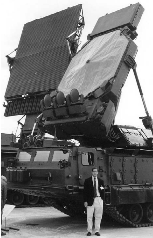
Figure 13.3 SA-12 Grill Pan fire control radar, with Bill Board surveillance radar in background [4].
