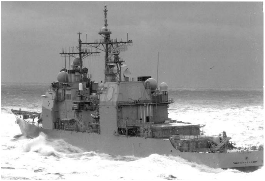
Figure 13.4 U.S. Navy Aegis cruiser, showing the aft/portside arrays of the AN/SPY-1 radar. (Figure courtesy of U.S. Navy.)
