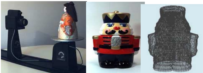
Fig. 17.1 (from left to right) Zoomage3D scanning device, a 1 ft tall nut-cracker toy and a 18,720 polygon mesh of the toy.
