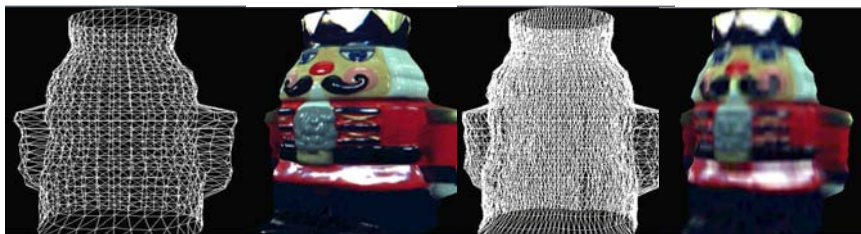
Fig. 9.5 Two representations of the Nutcracker texture+mesh models: Top has lower quality mesh, requiring 125 Kb total bandwidth, and higher perceptual quality; Bottom has higher quality mesh, resulting in lower quality texture to keep total bandwidth at 134 Kb, but has lower perceptual quality.
