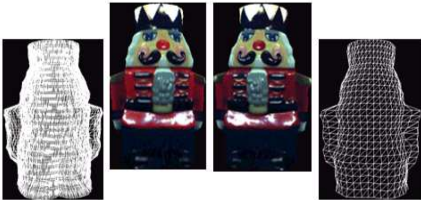
Fig. 6.1 The two nutcracker objects are perceptually similar although the mesh resolution on the left is ten times that on the right (18,720 vs. 1,872 triangles corresponding to 46 and 8 KB in .zip format).
