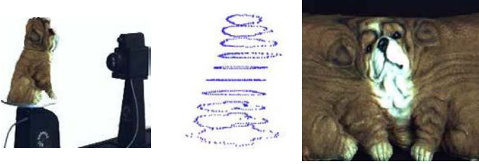
Fig. 5.3 (left) Zoomage 3D scanner and a dog object, (middle) sample of 3D scan-points, and (right) scanned texture image.
