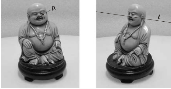
Fig. 12.13 Left and right images of a stereo pair: \ell is the epipolar line associated to p_1 .
