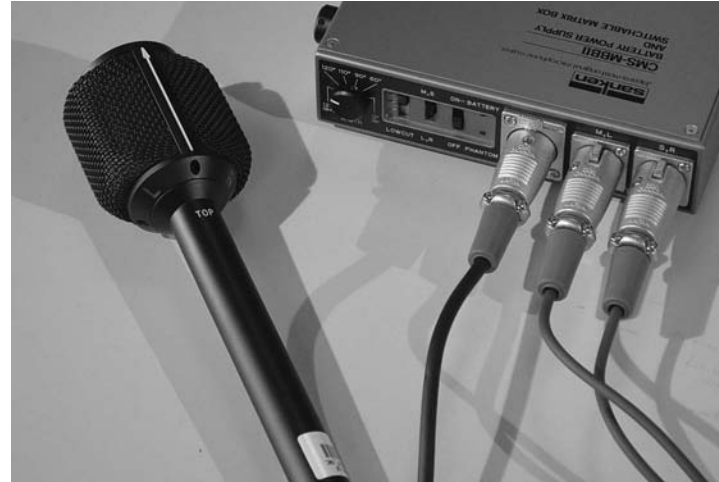
FIGURE 5.11. Middle/side stereo microphone.
