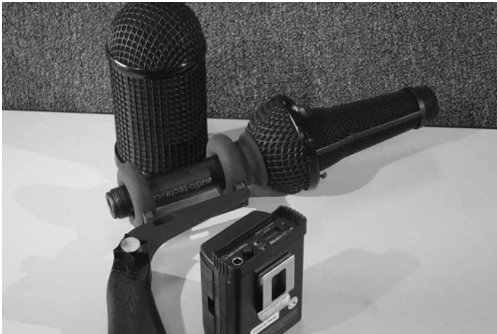
FIGURE 5.10. Adaptive array microphone.
