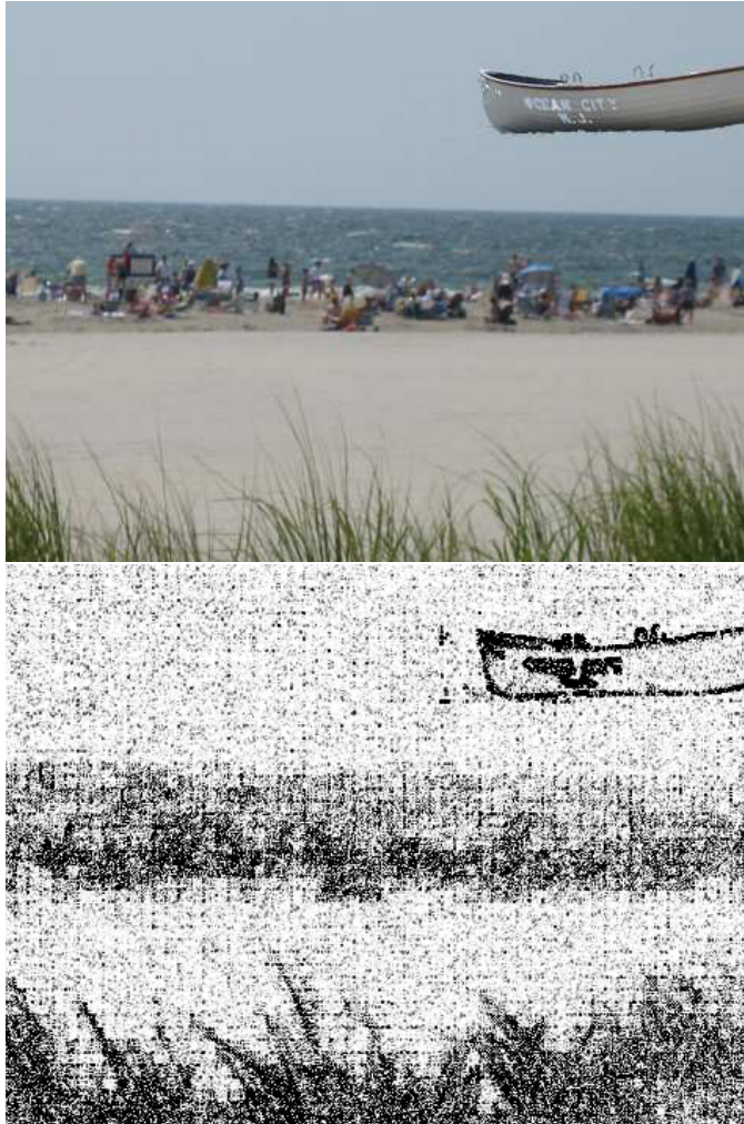
Figure 17.4: The upper image shows a photo of Ocean City, NJ modified by pasting a boat in the sky. The lower image is the output of Popescu and Farid's algorithm. The darkest spots are the ones where there's the most disagreement with the neighbors.
