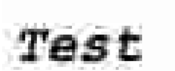
Figure 17.3: The JPEG compression function often leaves strong visual artifacts around hard edges. This image was created by compressing text with a very low quality, a process that encourages the artifacts by limiting the number of coefficients kept.
