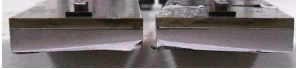
Figure A2-3 Inclined crack growth
