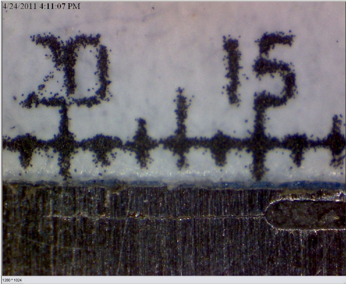
Figure A2-5 Notch and hair line crack in SE(T) specimens
