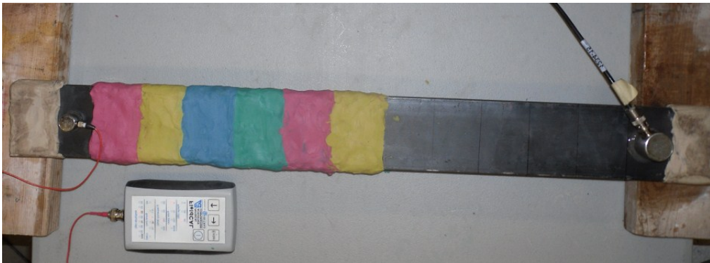
Figure A2-1 assessing the drop in Amplitude (Attenuation) in the specimen due to use of modeling clay
