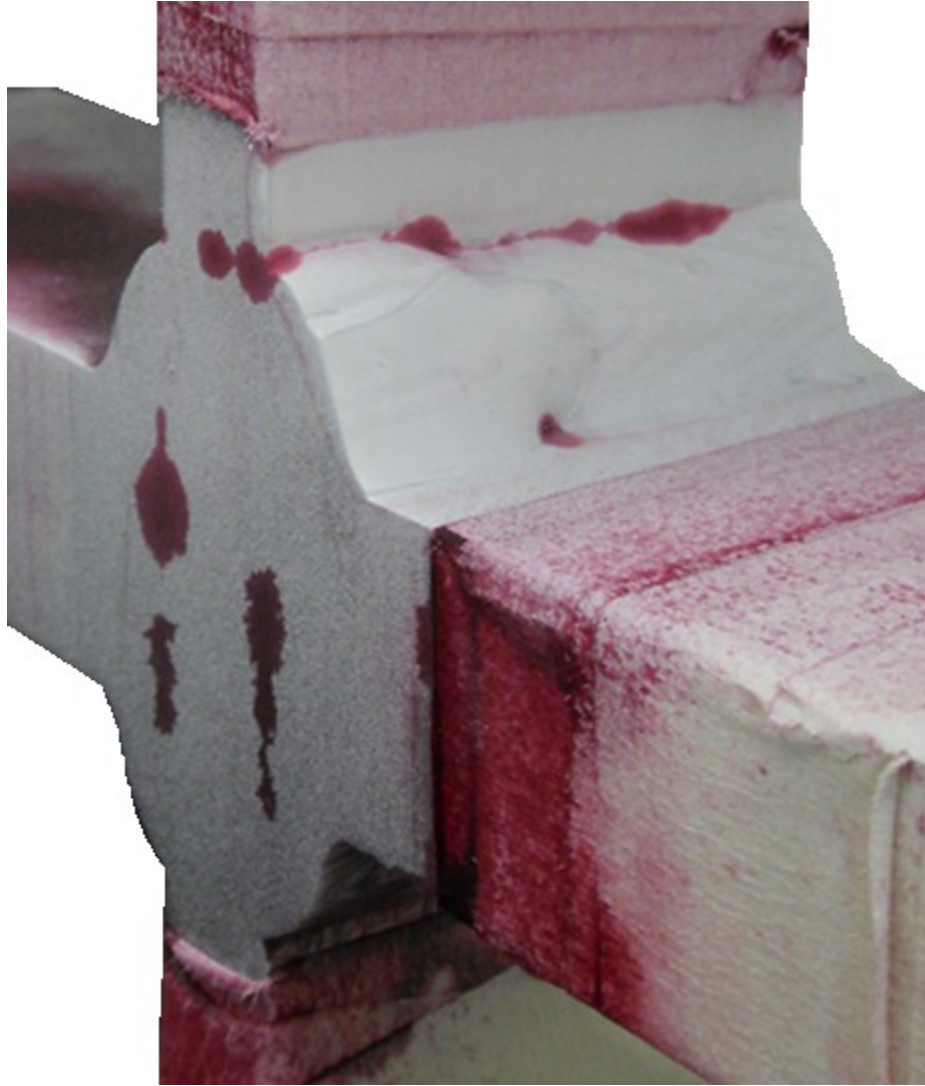
Figure A3-6 Specimen C6 - PT test 2
