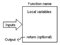
The large arrow represents the input pathway to the function, through its parameter list. The small arrow represents a single output from the function, generated as a result of a return statement. The two critical points are as follows:
