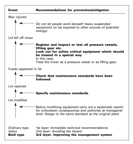
Figure 1.7 Summary of Section 1.2 - A mechanical accident
