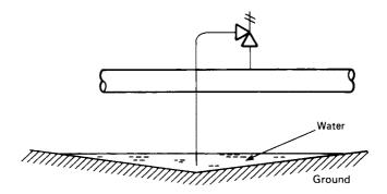
Figure 16.9 The end of the relief valve tail pipe was so close to the ground that it was below the surface of a puddle and was blocked when the puddle froze
