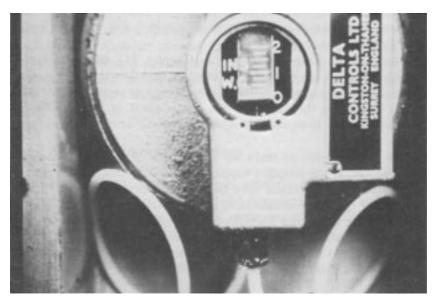
Figure 2.4 Note that on the switch, as shown here with the cover removed, the set-point has been reduced enough to disarm the protective equipment
