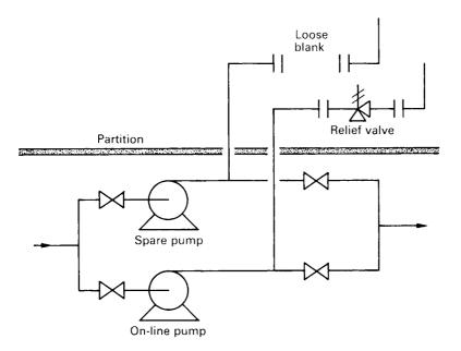
**Figure 17.2** Piper Alpha: the on-line pump broke down so the other pump, which was shut down for overhaul and for testing of the relief valve, was brought on line. The operators did not know that the relief valve had already been removed and the open end loosely blanked
