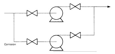
Figure 16.11 The lower pump was rarely used. Water collected and corrosion occurred
