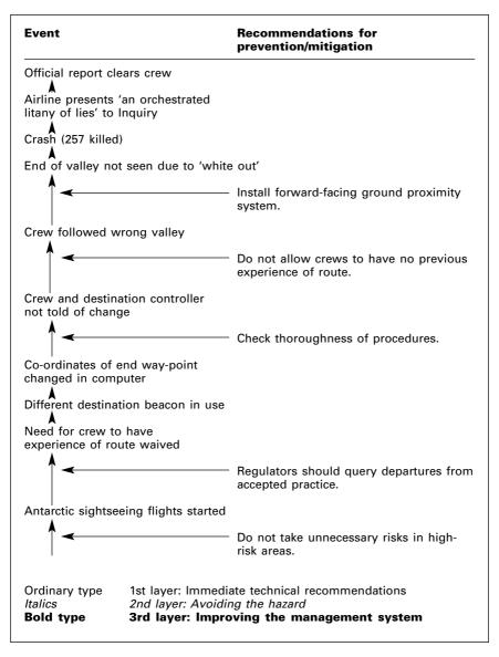
Figure 21.9 The Mount Erebus crash
