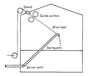
Figure 6.2 The tank was being splash-filled through a swing arm which was stuck in the raised position. (Drawing not to scale)
