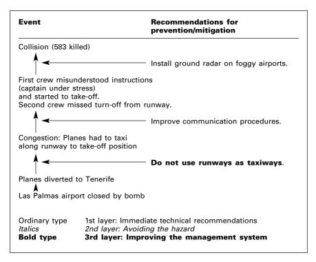
Figure 21.7 The Tenerife ground collision 1977
