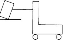
**Figure 15.4** Drums are lifted two at a time like this onto a flat wagon
