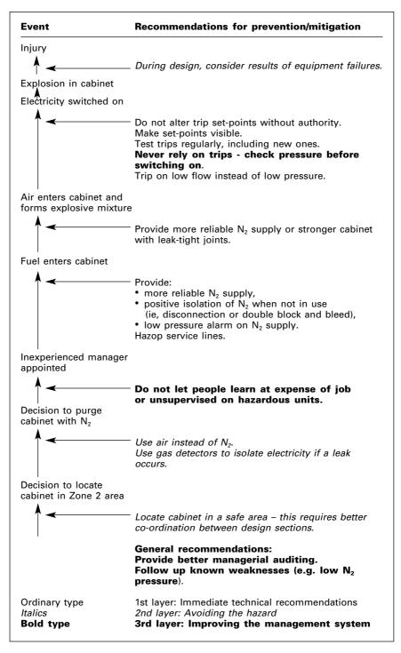
Figure 2.5 Summary of Chapter 2 - Protective system failure
