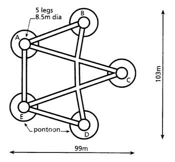
Figure 28.2 (a) The pentagon design of the Alexander Kielland offshore rig (Reproduced with permission from Macmillan<sup>3</sup>)
