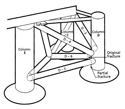
Figure 28.2 (b) Close-up of columns C, D and E showing bracing (Reproduced with permission from Macmillan<sup>3</sup>)
