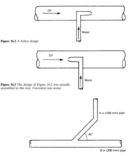
Figure 16.4 A poorly designed joint which failed, causing a major leak
