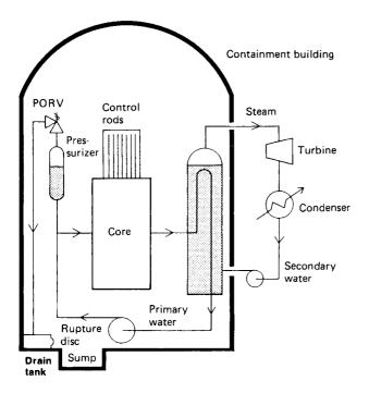
Figure 11.1 A pressurized-water reactor - simplified
