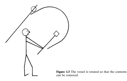
It was then found that the welds between the lid and its hinges had cracked. It was a fatigue failure, caused by the strains set up by repeated opening and closing of the lid. There was nothing wrong with the original design but the lid had been modified about ten years before the incident occurred and, in addition, some repairs carried out a few years before had not been to a high enough standard.
