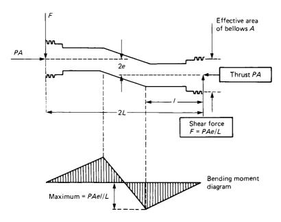
**Figure 8.2** Sketch of pipe and bellows assembly showing shear forces on the bellows and bending moments in the pipe (due to internal pressure only). (Reproduced by permission of the Controller of Her Majesty's Stationery Office)
