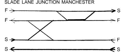
Figure 23.1 An example of railway track which requires conflicting train movements. The layout has now been changed. F = fast, S = slow
