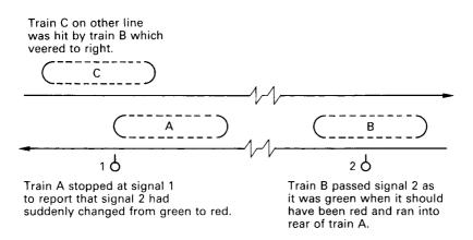
Figure 19.2 The Clapham Junction railway accident
