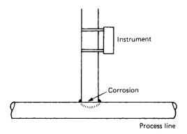
Figure 16.12 Water collected in a piece of pipe, used as an instrument support, and corrosion occurred
