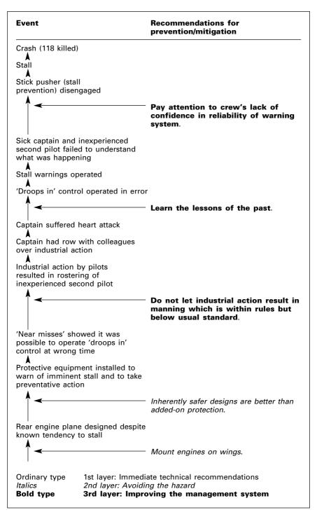
Figure 21.4 The Trident crash at Heathrow 1972
