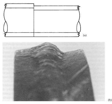
Figure 16.5 (a) and (b) Two pipes of slightly different diameter were welded together
