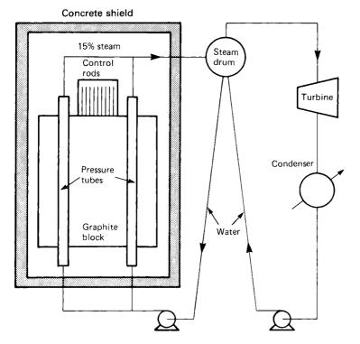
**Figure 12.1** The Chernobyl reactor, simplified. The fuel is contained in 1661 zirconium alloy pressure tubes set in a graphite block. Water passes through the tubes. There are over 200 control rods
