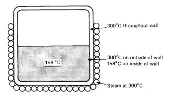
Figure 9.1 The Seveso reactor. The hot upper portion of the reactor wall heated the surface of the liquid
