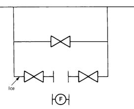
Figure 16.10 When the flowmeter was removed it formed a dead-end in which water collected
