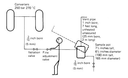
Figure 7.4 An attempt to clear a choke and obtain a sample from the line joining two reactors
