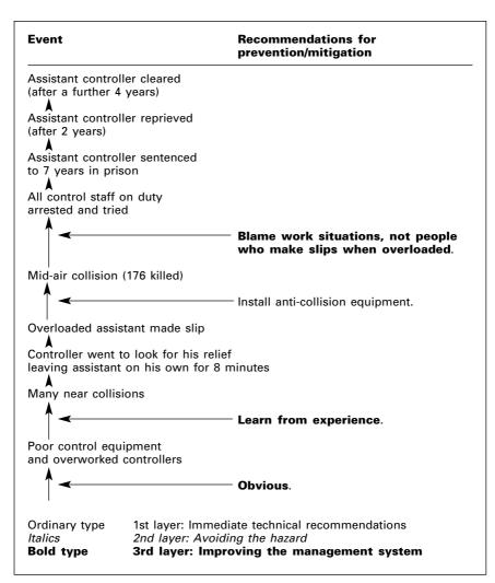
Figure 21.6 The Zagreb mid-air collision 1976
