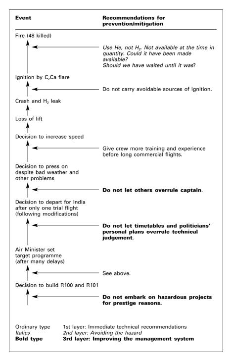
Figure 21.1 The R101 airship disaster 1930
