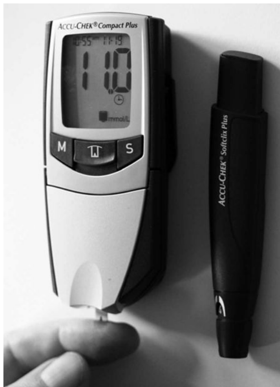
Figure 18.7 A biosensor for glucose used in diabetes monitoring. A drop of blood is applied to the disposable electrode at the bottom with its glucose concentration being produced on the read-out a few seconds later. On the right is a system for the controlled pricking of a finger.
