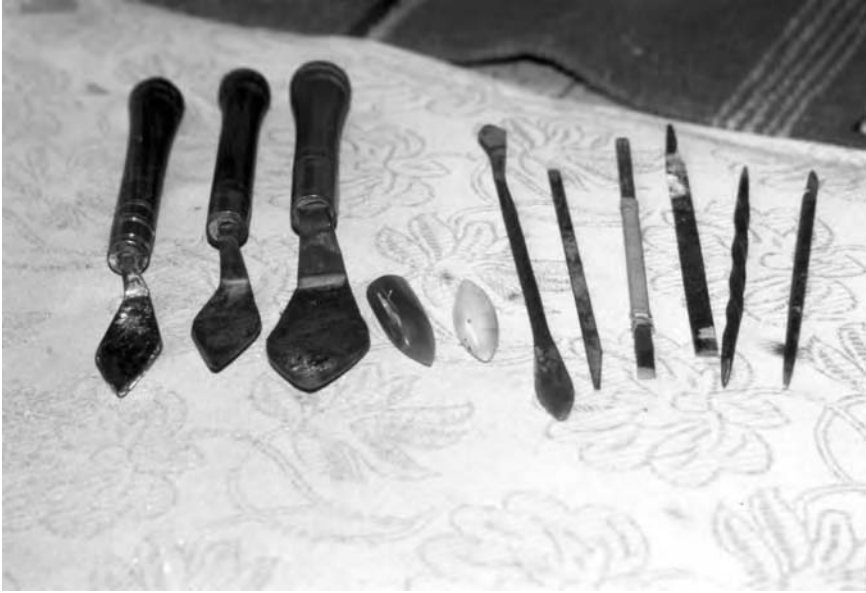
Figure 7.4 Tools used in traditional mural painting: trowels of different size, pieces of agate stone and other implements.
