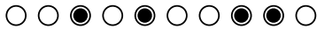
Fig. 1.3 Ten atoms that can accommodate four quanta of energy. An atom with a single quantum of energy is shown as a filled circle, otherwise it is shown as an empty circle. One configuration is shown here.
