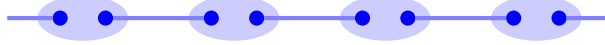
Fig. 4.3 A Valence-bond Solid. Each blue dot denotes a spin-1/2 particle. Each solid line connecting two particles are called a ‘bond’, which represents a singlet state. Each oval contains two particles, which represents the projection of those two particles onto the spin triples subspace
