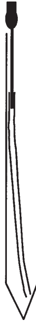
Fig. 2. Hypodermic needle with a piece of polyethylene tubing attached in a 15-mL plastic tube.
