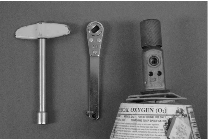
FIGURE 1.3 Cylinders are opened and closed either using a ratchet spanner (left), cylinder key (centre) or hand-operated valve (right).
