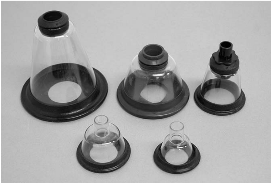
FIGURE 1.10 Face masks for use with a range of laboratory species. The rubber diaphragm helps provide a better seal around the animals nose (F-042).
