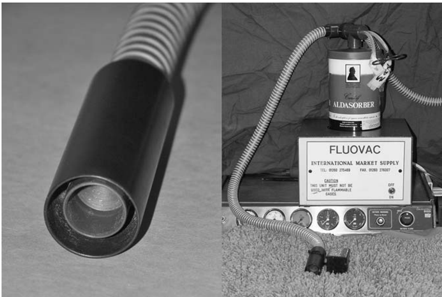
FIGURE 1.11 Concentric mask system for rodents and rabbits that combine delivery of an anaesthetic gases with removal of waste gas through an outer tube. An extraction fan and activated charcoal absorber are used to remove the anaesthetic gases and prevent exposure of personnel (Harvard Instruments).
