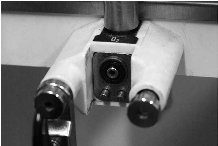
FIGURE 1.1 Pin index system – the pins in the mounting block (left) fit into the holes in the gas cylinder (see Fig. 1.3).
