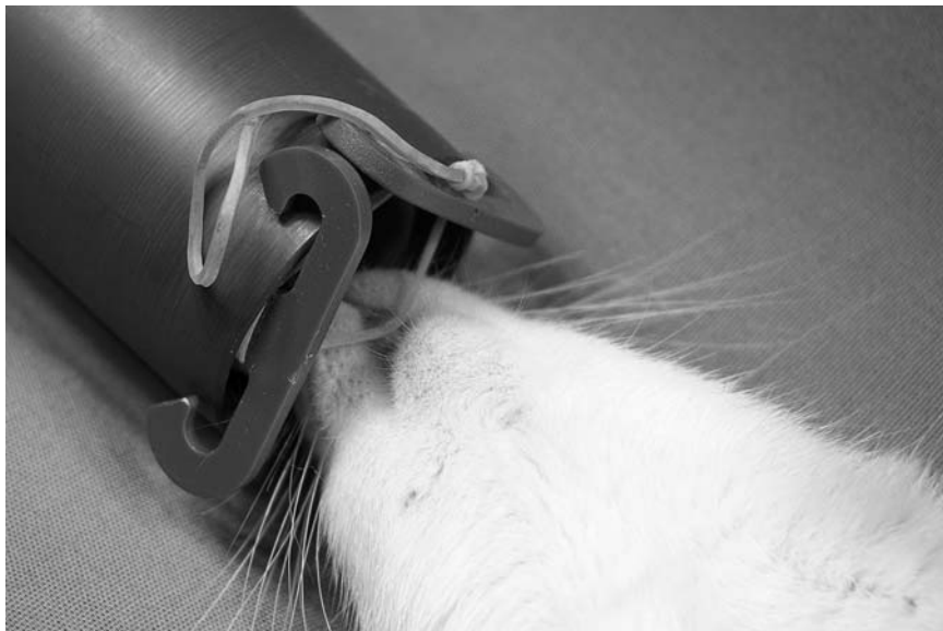
FIGURE 2.12 Elastic band used to help maintain the position of a rat or mouse in a face mask. The attachment is made from the components of a protective face mask (Segre, Sweden). (Concentric mask supplied by VetTech Solutions.)
