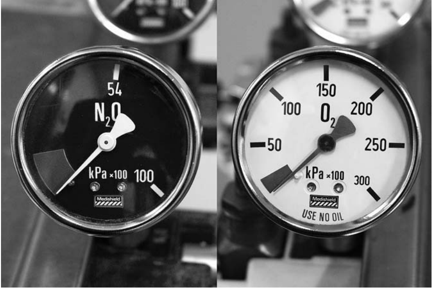
FIGURE 1.2 Pressure gauges for nitrous oxide (left) and oxygen (right) cylinders.
