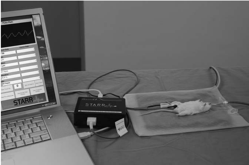
FIGURE 3.3 The ‘Mouseox’ pulse oximeter in use. The system both provides pulse oximetry data and records respiratory rate by processing of the pulse pressure data. The instrument does not require positioning as closely to the animal as shown in this illustration (Y-27).
