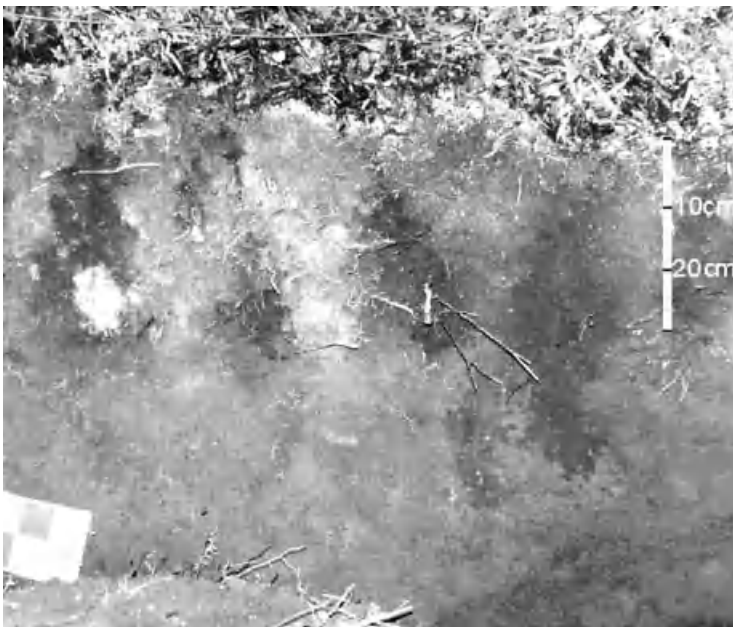
Figure 1.1 Staining by dye after infiltration at the soil profile scale in a forested catchment in the Chilean Andes (from Blume et al., 2009).
