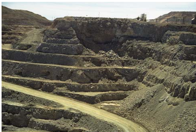
Fig. 20. Remining of an abandoned underground gold deposit in the Kalgoorlie/Western Australia Super Pit by daylighting through Kalgoorlie Consolidated Gold Mines. Some of the old mine workings can be seen in the middle of the photograph. The remining contributes to a reduction of the pollutant loads as potentially acidic strata are excavated, processed and disposed of.
