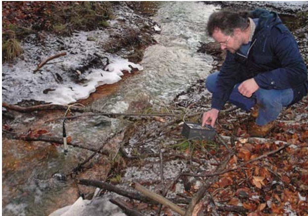
Fig. 61. Flow measurement with the salt dilution method in the turbulent Gernrode/Harz/Germany Steinbach Creek. The salinity probe is hanging in the middle of the stream and the data logger records the electrical conductivity every second (photographed by Andrea Berger).
