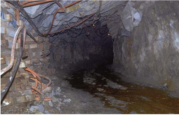
Fig. 17. Unflooded access Gallery in the Western Deep Level/South Africa underground mine. The Gold Reef comes in from the top right side and dips to the lower left corner. Concrete support helps to support the geomechanical stability in the 2500 m deep gallery.
