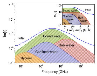
**Figure 2:** Dielectric response of the 19.69 mol % glycerol-water mixture in the frequency range from 50 MHz to 0.5 THz reflecting the complexity of glycerol-water interactions. The imaginary and the real (in the inset) components of the dielectric spectra have been decomposed in to four relaxational processes with different relaxation time constants.
