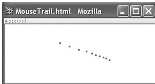
FIGURE 5.17 Trail of blips marking the last 10 locations (as recorded by mousemove events) of the mouse cursor.
