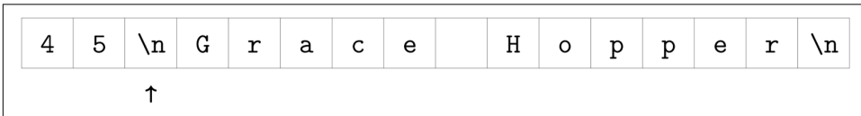
Figure 3-4. A stream of characters after nextInt is invoked.
