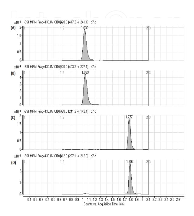
Figure 2. LC-MS/MS chromatogram in MRM mode for metabolite (BPAG) and parent bisphenol A (BPA) of a typical microsomal incubation. (A) mass transition for BPAG<sub>d16</sub> (internal standard for BPAG), (B) mass transition for BPAG, (C) mass transition for BPAd16 (internal standard for BPA), (D) mass transition for BPA. For analysis conditions refer to [4].
