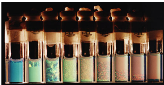
Fig. 3.4 Dispersions with hard-sphere like PMMA spheres at volume fractions around the fluid–solid phase transition. From Pusey and Van Megen [9]. Samples are denoted from left to right as samples a, b,... i. See Fig. 3.5 for the state of each sample. Picture reprinted from Pusey and Van Megen [9], Copyright 1986, with permission from Nature. Kindly provided by P.N. Pusey
