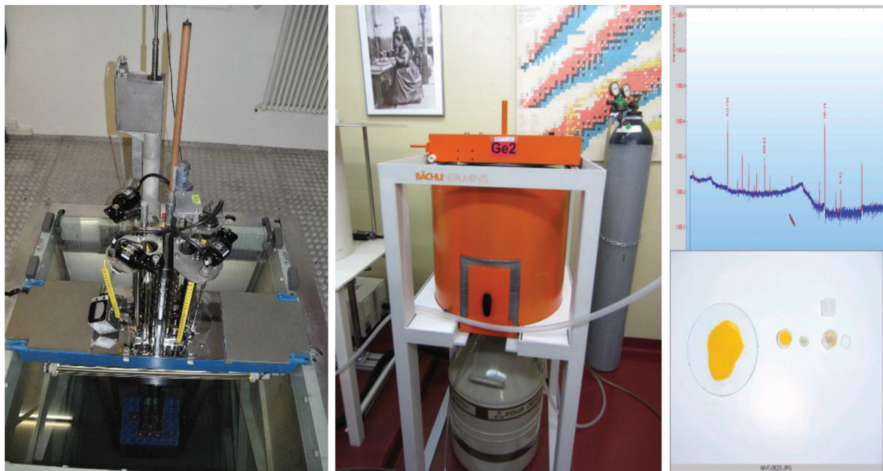
Figure 1. Equipment for NAA. Swimming pool reactor (left) gamma-ray spectrometer with lead shielding (middle) gamma-ray spectrum (above right) curry sample and sample device for the irradiation [4].
