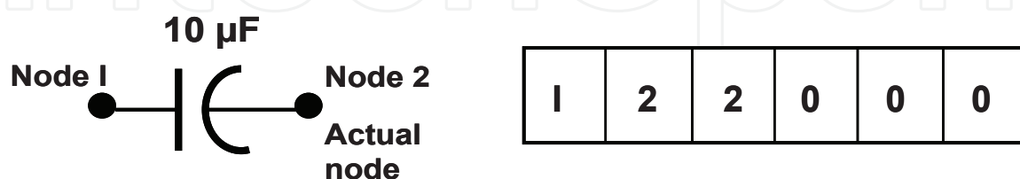
Fig. 8. An element of circuit and its corresponding gene.
