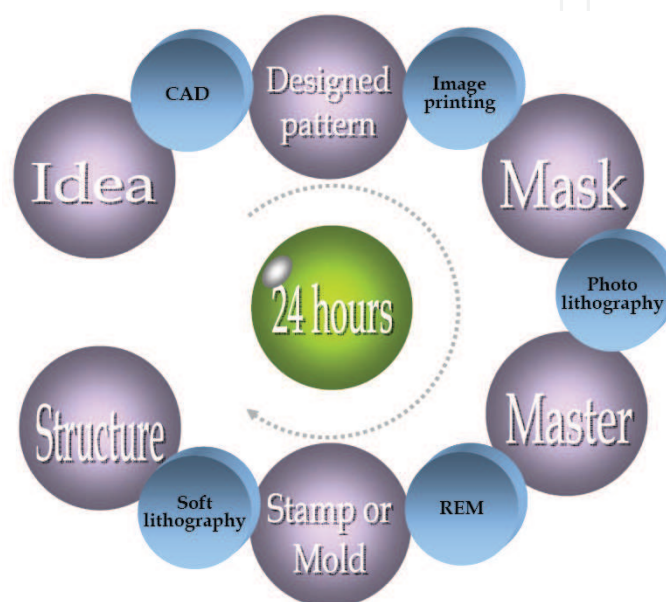
Fig. 2. The rapid prototyping procedure for soft lithography.
