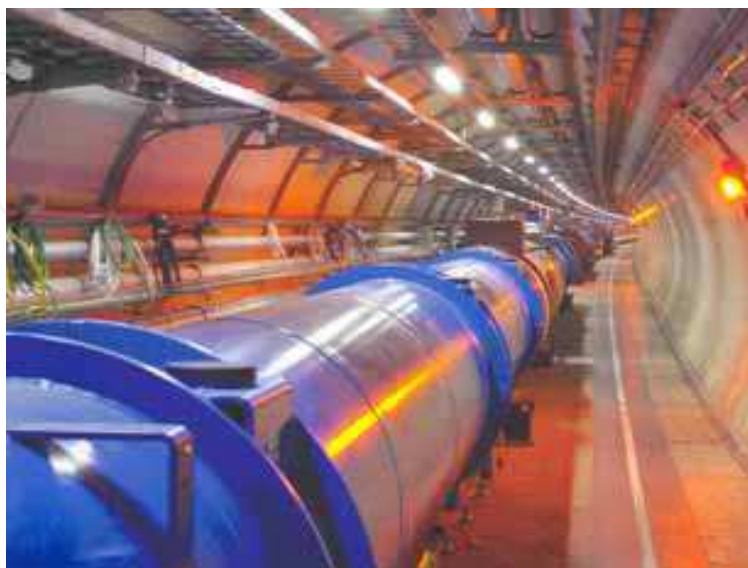
Fig. 24. 1232 superconducting dipoles for Large Hadron Collider (After Rossi, 2006).
