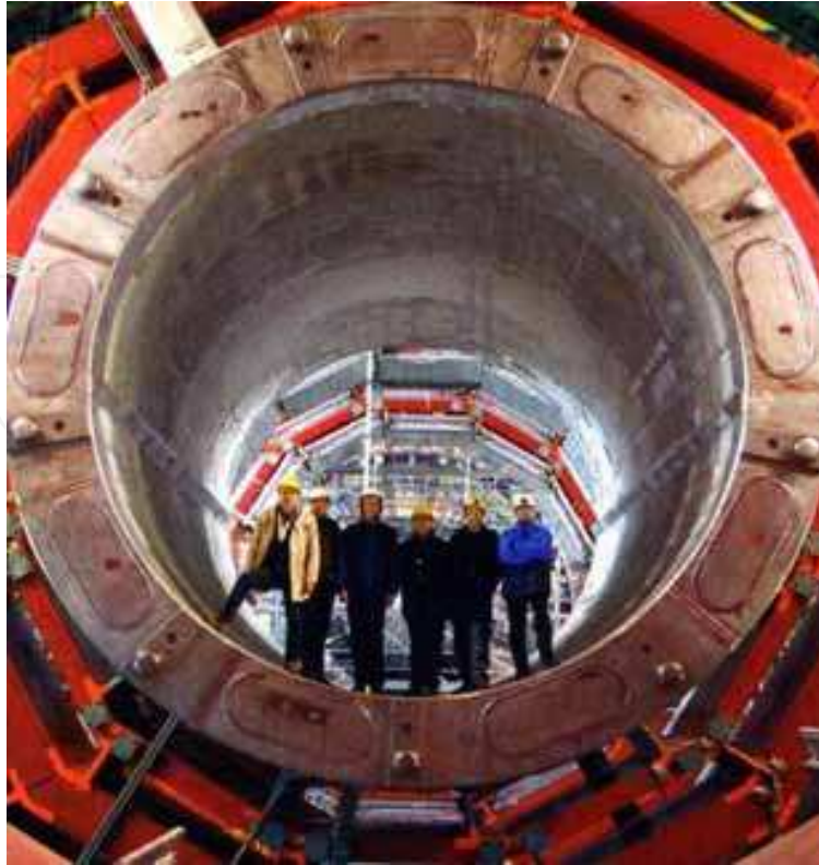
Fig. 25. Superconducting solenoid for the Muon Spectrometer (Barney & Lee, 2006).
