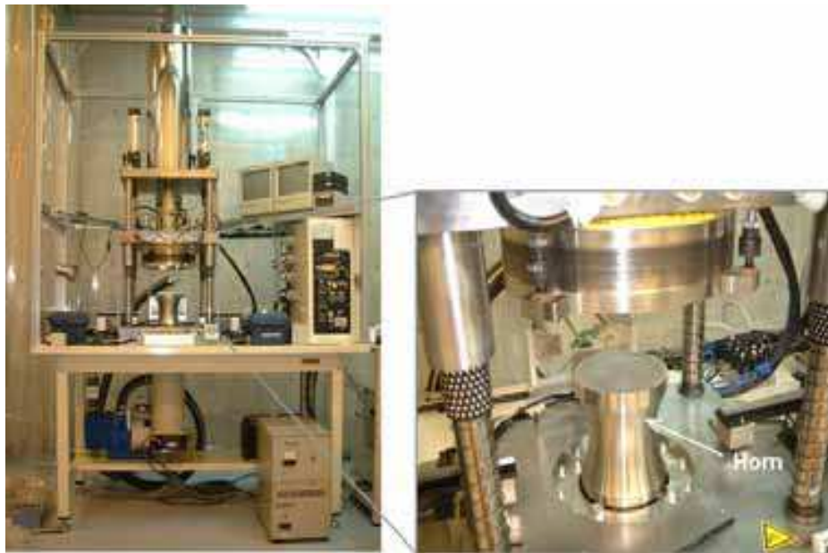
Fig. 2. (a) Photograph of an ultrasonic hot embossing system, and (b) bottom loading stage based on an ultrasonic horn.
