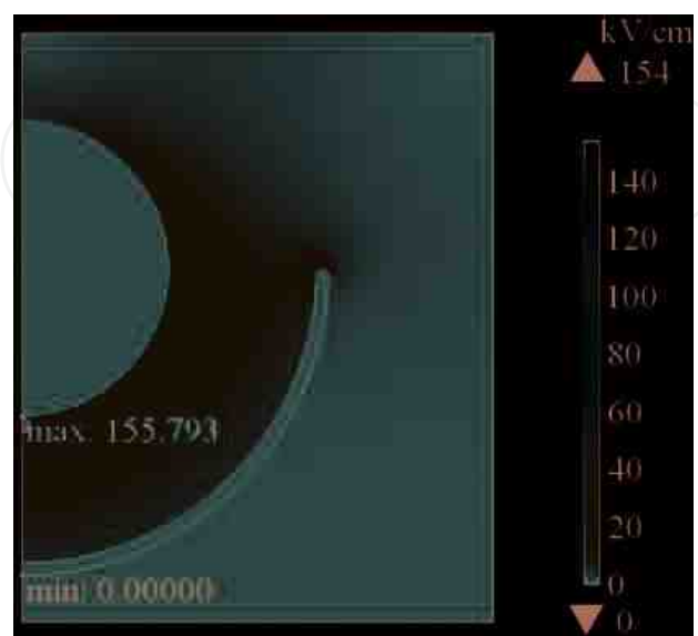
Figure 8. P-type insulation defect space electric field simulation output.
