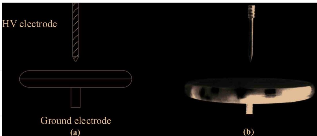
Figure 3. N-type insulation defect model. (a) Model diagram and (b) physical diagram.
