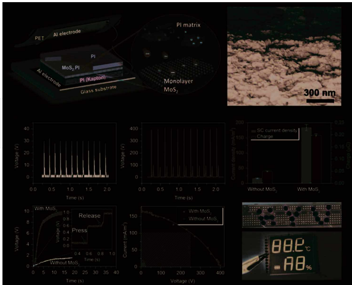
Figure 4. A contact-separation mode TENG with monolayer MoS 2 [21].
