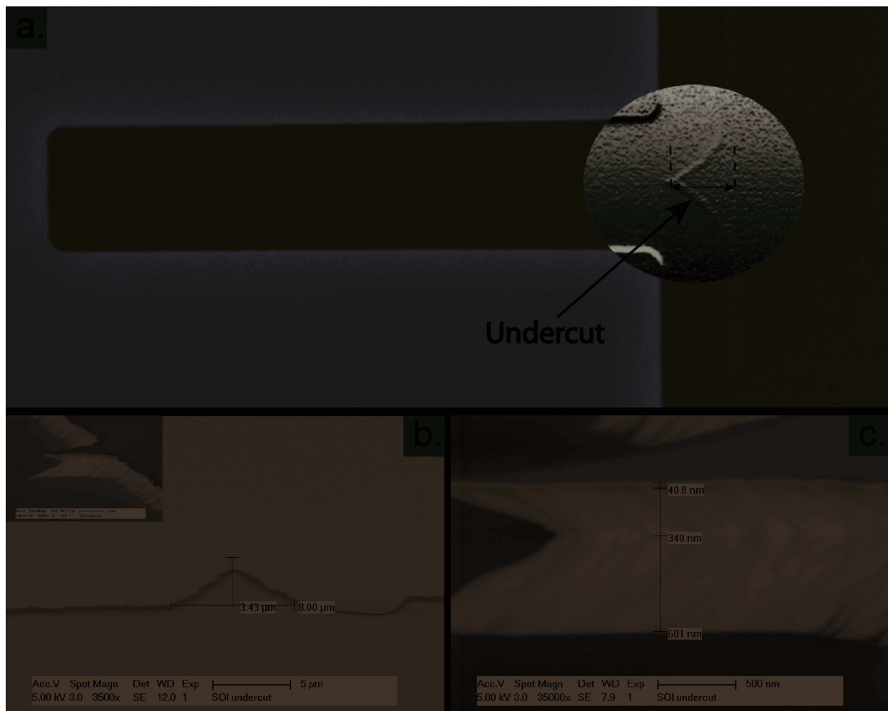
Figure 6. (a) Optical microscope image of a cantilever with hidden anchor due to under etching of the base of the cantilever. (b) SEM of a hidden anchor. The cantilever was forcibly removed in order to see the hidden anchor. The inset shows the bonding surfaces of the SOI wafers were in the middle of the BOX layer. (c) Close-up view of bonding interface and silicon device layer.
