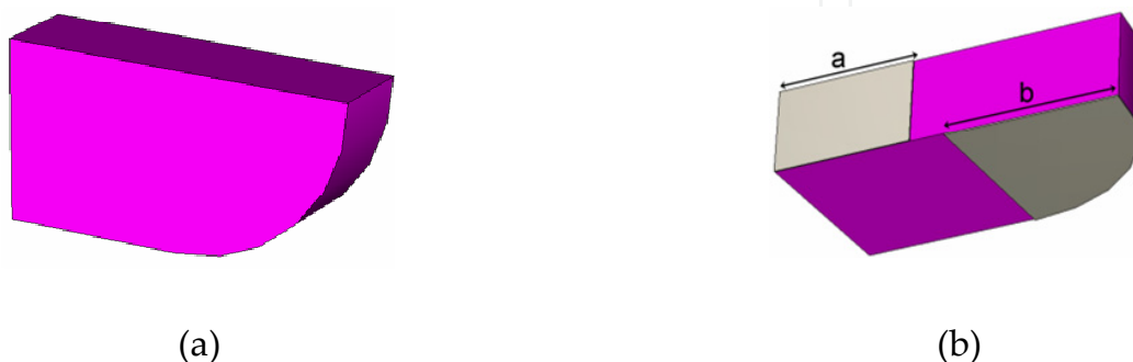
Figure 19. Proposed DR shape (a) and metallization of two different sides (b)
