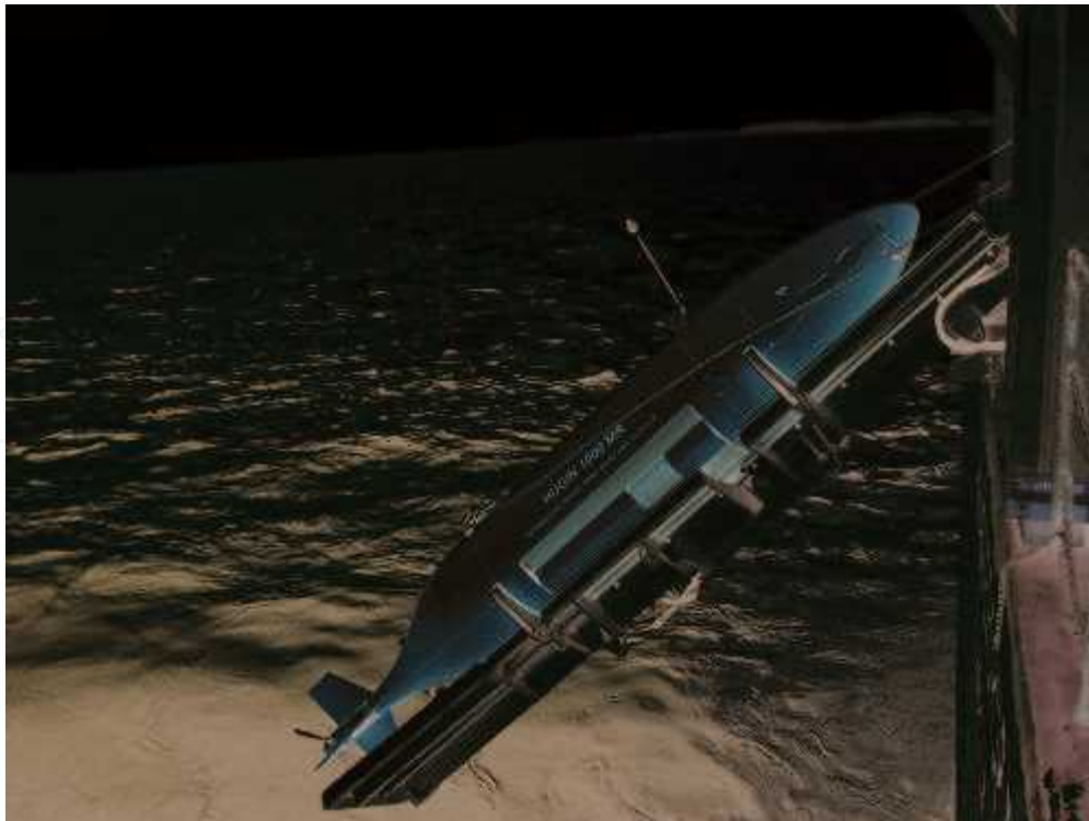
Fig. 15. The HISAS 1030 interferometric SAS on the HUGIN autonomous underwater vehicle. The picture was taken just before launch during a scientific mission on board the research vessel H U Sverdrup II in Norwegian waters in April 2010.
