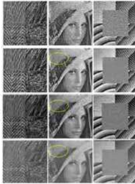
Fig. 16. A comparison of the visual aspect of the results of three despeckling methods; From up to bottom: noisy sub-images, results obtained applying the method in [Walessa&Datcu, 2000], results obtained applying the method in [Ifremer, 2010] and results obtained applying the method based on the HWT.
