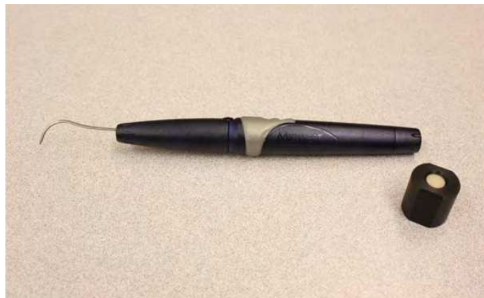
Fig. 9. Midwest Caries I.D. device and the standard for calibration procedure.
