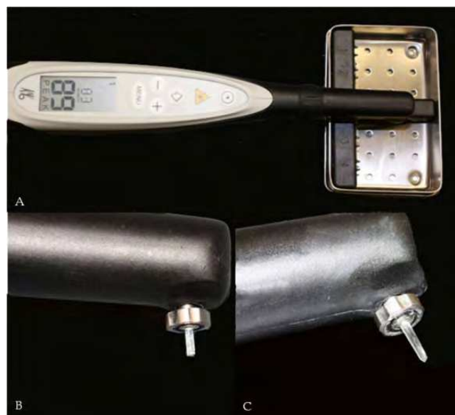
Fig. 6. (A) DIAGNOdent 2190 or DIAGNOdent pen calibration against the standard ceramic. (B) Occlusal tip. (C) Approximal tip.
