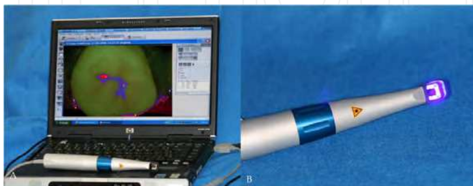
Fig. 8. (A) VistaProof fluorescence camera and DBSWIN software analysis. (B) Six blue LEDs emitting a 405-nm light.
