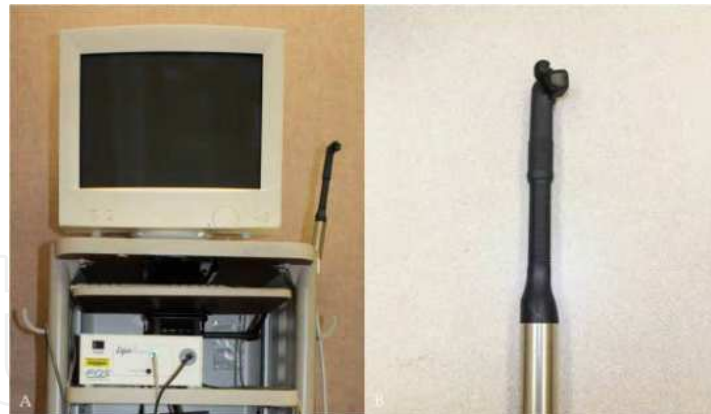
Fig. 11. (A) Digital imaging fiber-optic transillumination (DIFOTI). (B) Tip for occlusal surfaces.
