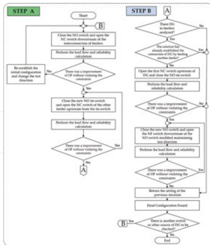
Figure 7. Flowchart from step A and step B of heuristic search technique for reconfiguration of distribution networks.
