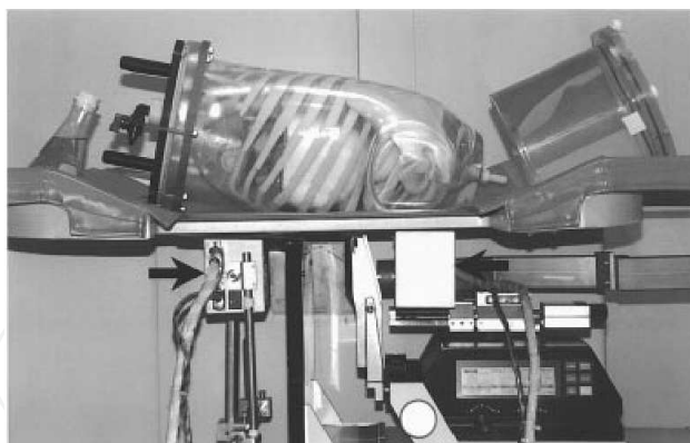
Figure 7. Image of the West Virginia University - Jefferson Laboratory PEM system. The PEM detector heads, mounted in a biopsy table, are highlighted by the black arrows. A torso phantom can be seen in the table. From [27].
