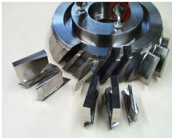
Fig. 26. Pre-machined BLISK demonstrator, after extraction of blade-blocks.
