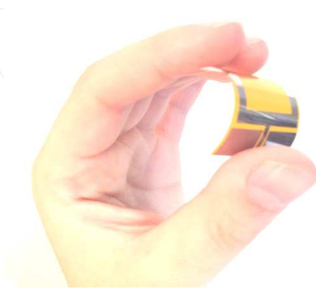
Figure 1. Flexible printed monopole antenna based on Kapton Polyimide substrate.
