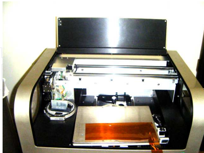
Figure 8. Installing the polyimide substrate on the platen of the material printer.
